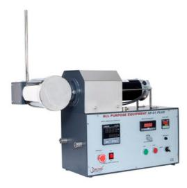
Ball mills can be used for crystalline material. A ball mill is useful for mixing dry materials and under certain conditions wet material. The ball mill jar is made of complete stainless steel 304. The diameter of S. S.ball varying between 10 mm to 30 mm is provided with a ball mill. The ball mill can be attached to the main drive through the universal gearbox.
