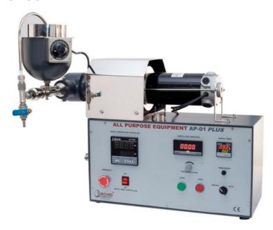
This unit is suitable for mixing of different types of liquids like emulsions (oil in water & water in oil). A piston pump produces homogenization. The vessel is made of S.S. 304 material and the vessel is jacketed with heating element which controls the temperature of material inside vessel thermostatically.
